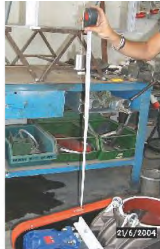
7349 Impact test for case hit on the side
