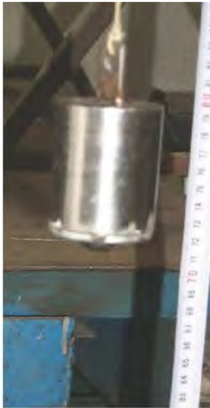
7348 Impact test at 0.7 metres (1Kg steel mass with d.25 sphere)
