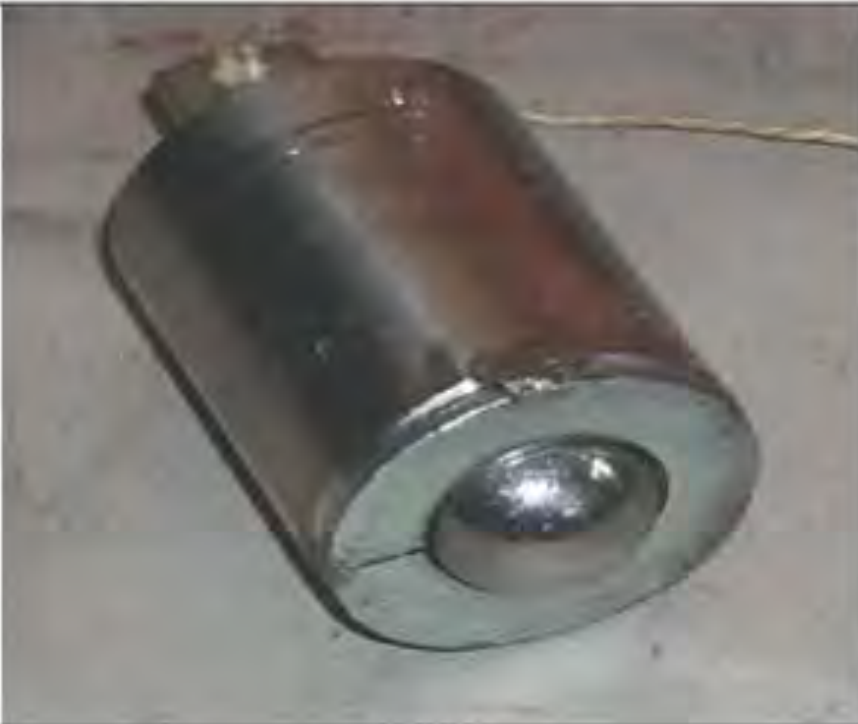
7333 Impact test 1Kg steel mass with d.25 sphere
